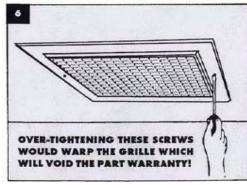
Use ½" grille mounting screws and predrilled holes to mount the ceiling grille into position on the vent.
