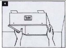
Being careful not to damage the aluminum lid, slide the vent into the ceiling opening – with the hinged end toward the outside house wall.
