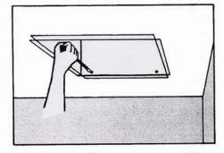
can be formed from a wire coat hanger, check to be certain you will avoid any attic obstruction within the 12" minimum attic clearance limit.
