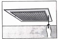
and away from the ceiling joist a distance of 11-5/8". Then, recheck all of your measurements and right angles and scribe the cutting lines. Now, cut out the square. (Height of ceiling insulation around the opening MUST NOT EXCEED 6".)
