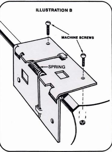
3. Next, referring to illustration B, loosely mount the aluminum barometric damper lid. With the LID HINGE BALANCING SPRING in position, tighten the machine screw nuts. HINT: If either of the front lid corners does not seat reasonably well on the rubber gasketing, carefully "tweak" UPWARDLY the diagonally opposing hinge-end lid corner (as is done—if or when necessary—on final quality control inspection of Mission's factory-assembled Up-duxe ceiling vent models).
