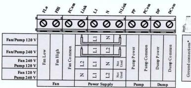
\*<u>Note</u>: Use a suitable wire connector (eg wire-nut) to terminate all ground connections for power supply, fan, pump, dump and cooler cabinet.
